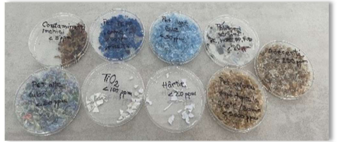
Contaminants from HWF - materials rejected during sorting process based on laser spectroscopy
